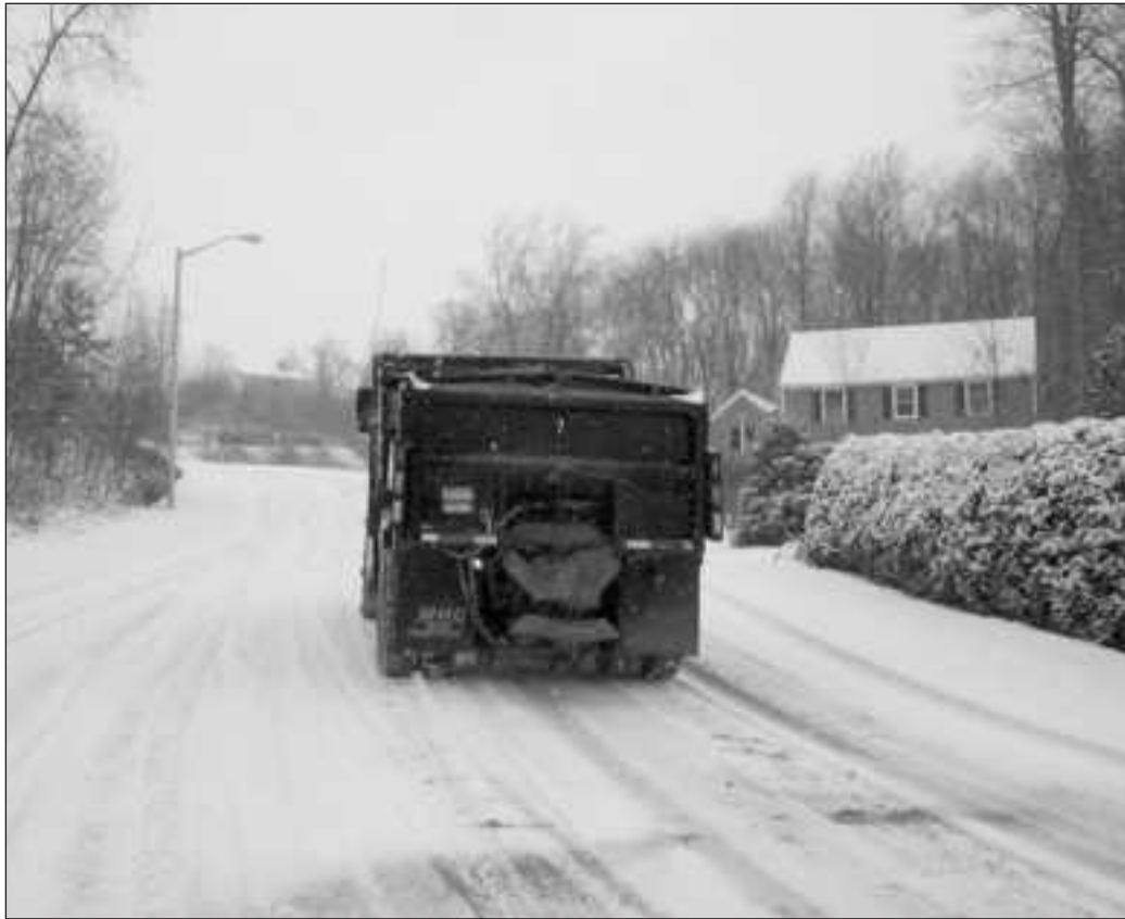
Marlborough uses a mixture of salt and abrasives for anti-icing and deicing.
